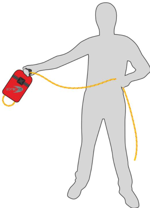
Throwlines are usually best delivered underarm and beyond the victim. This provides greater accuracy and is preferred option when deployed near overhead hazards i.e. trees or power lines.
